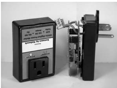
Fig. 2 Integrated ES02 module with the plug-in case
